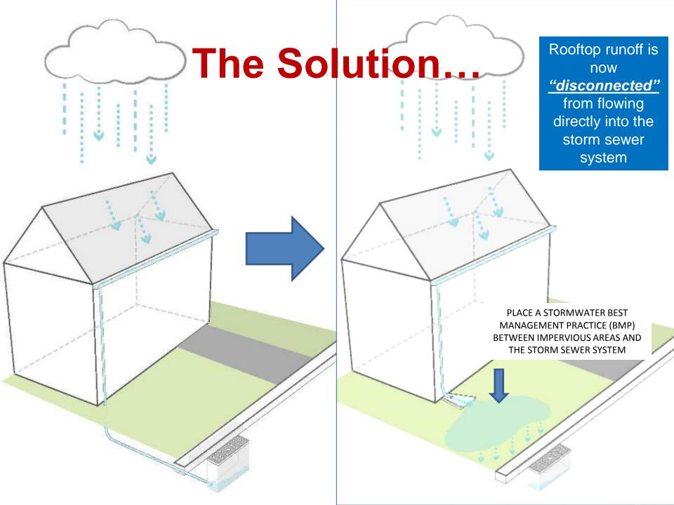
For 1.25 inch storm, 3,811 cubic feet of runoff = **28,500 gallons**
