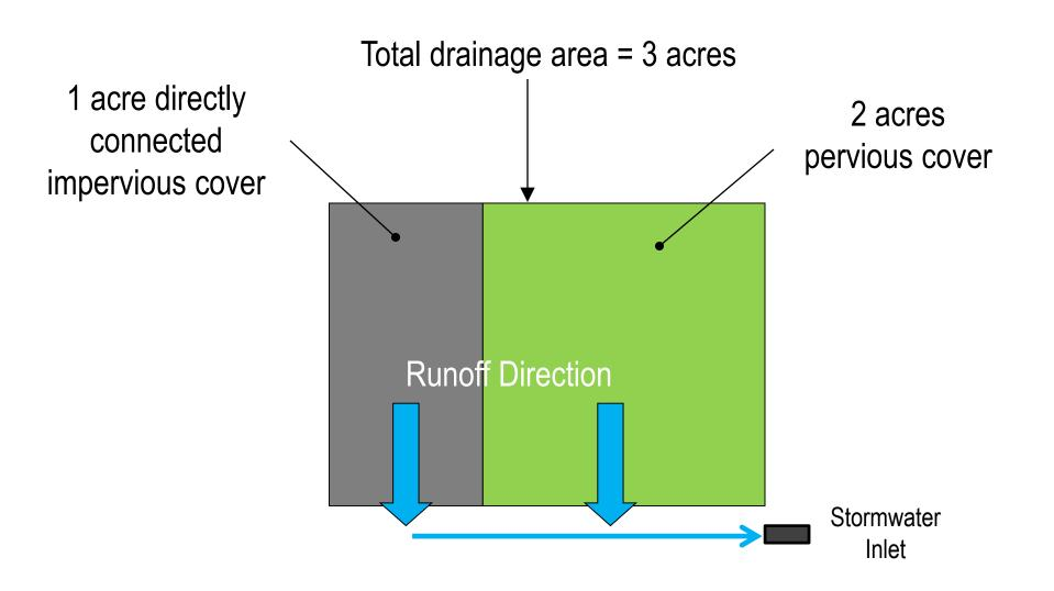
For 1.25 inch storm, 581 cubic feet of runoff = **4,360 gallons**
